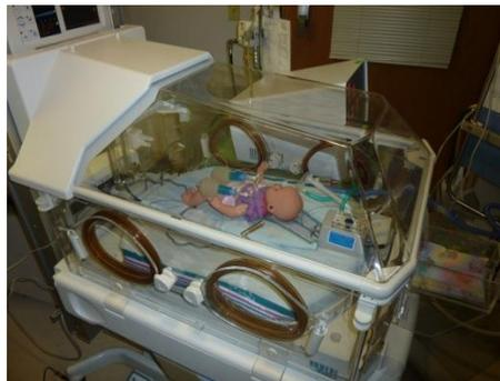
**Figure 1:** *Instrumented baby inside incubator with artificial lungs.*
