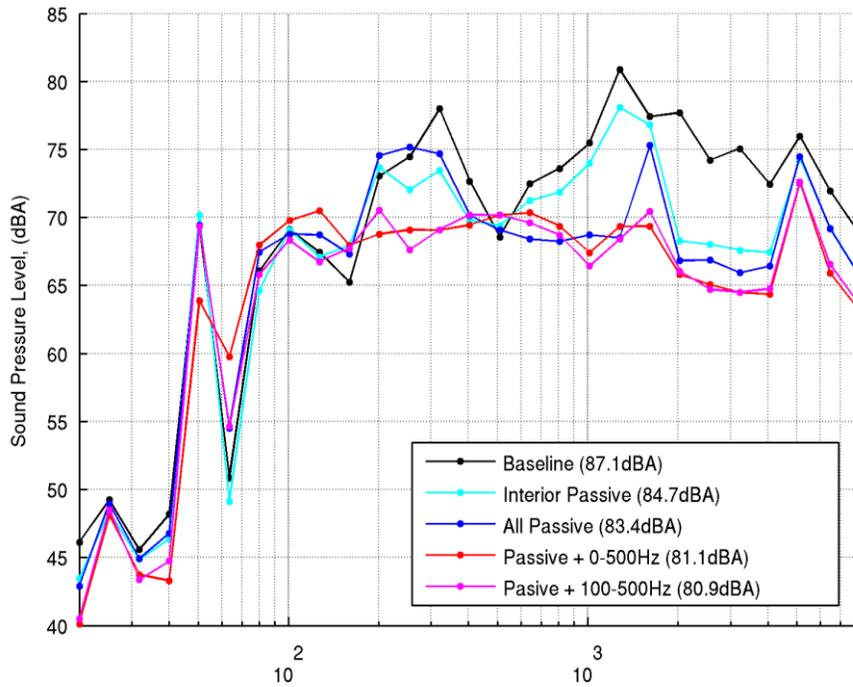
**Figure 11:** Treatment and active control performance (mean of four monitor microphones in  $1/3^{\text{rd}}$  octave bands).
