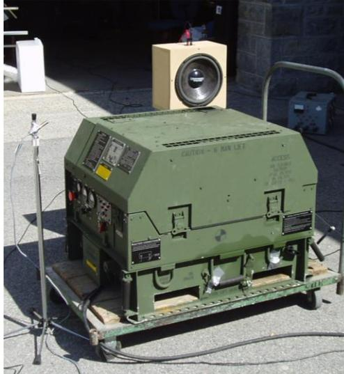
**Figure 1:** Photograph of 3kW generator with example prototype ANC source.
