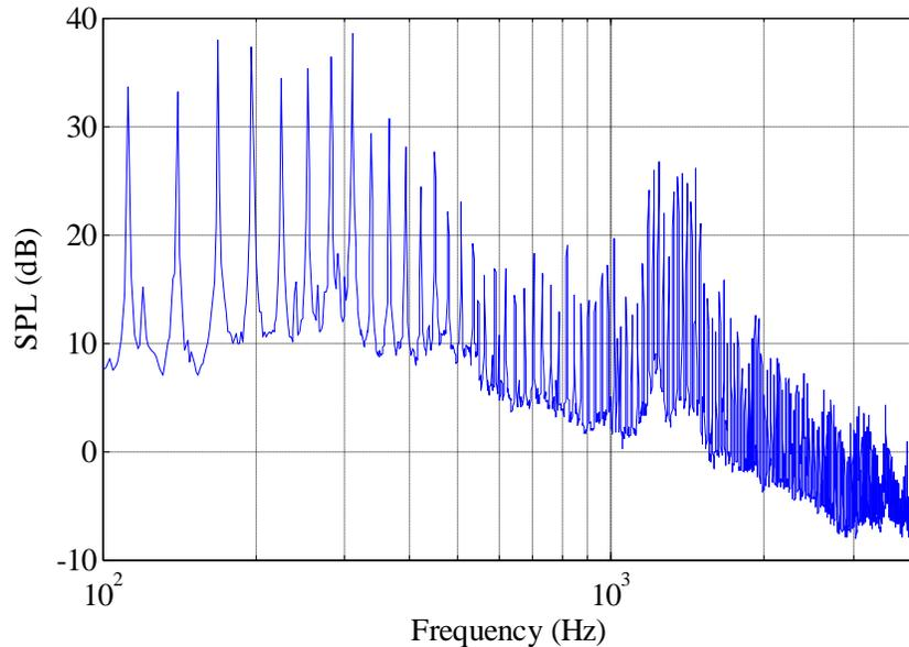
**Figure 3:** Average microphone spectrum for the array in front of face 2.
