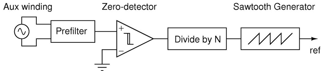
**Figure 7:** Pseudo-schematic of reference generation circuit.
