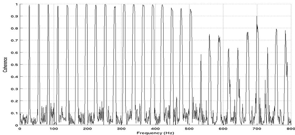
**Figure 8:** Measured coherence between reference signal and far field microphone.
