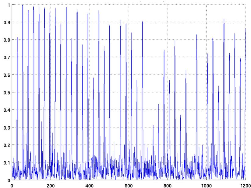
**Figure 5:** Coherence between far field microphone and accelerometer on cylinder head.
