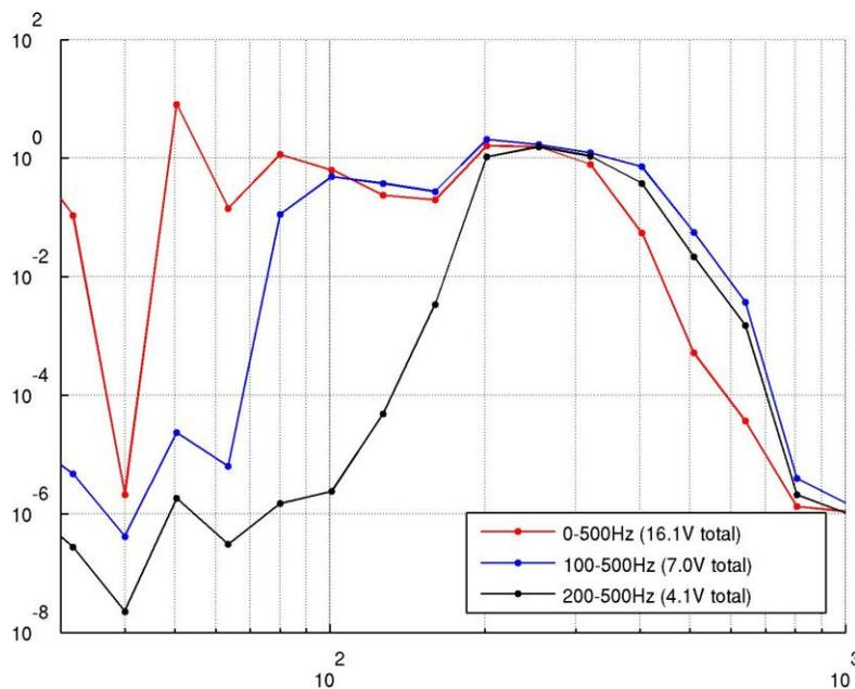
**Figure 12:** Speaker voltage filtered in  $1/3^{\text{rd}}$  octave bands.
