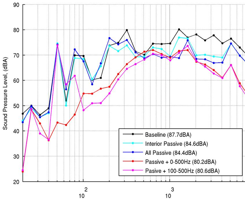
**Figure 10:** Treatment and active control performance (error microphone in 1/3<sup>rd</sup> octave bands).
