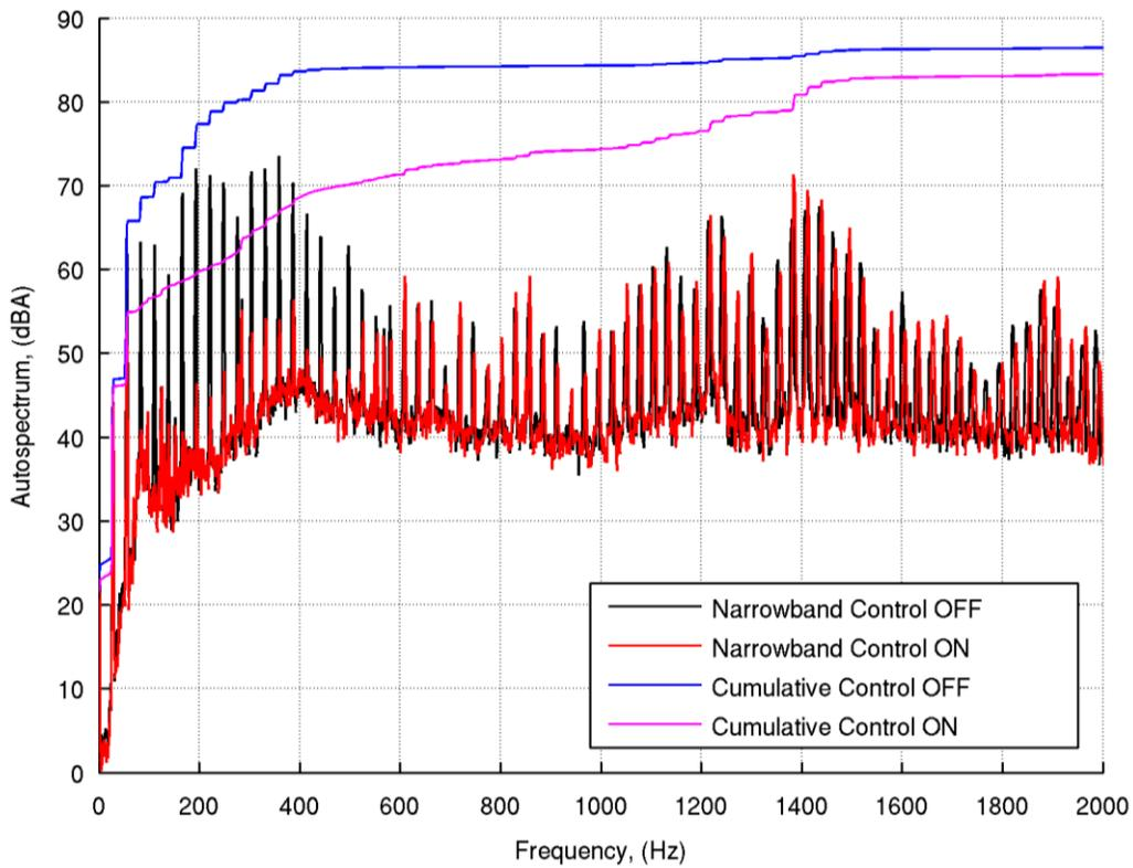
**Figure 9:** Narrowband and cumulative integral spectral plot of error signal with and without active control.
