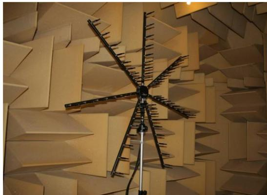
**Figure 2:** Photograph of the 63-element microphone phased-array.
