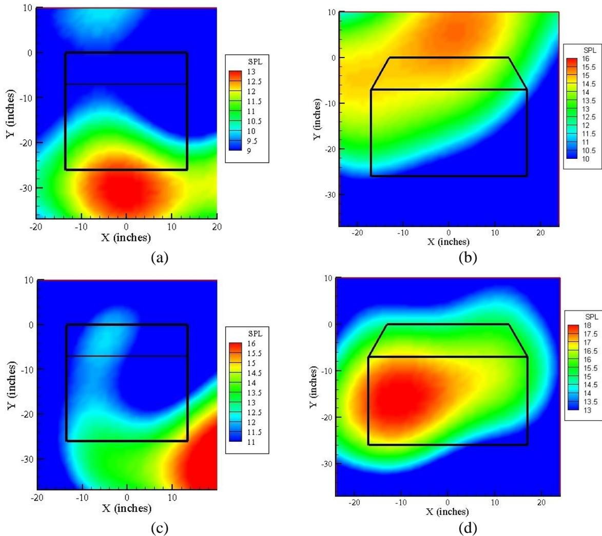
**Figure 4:** beamforming maps of (a) face 1 at 1394 Hz, (b) face2 at 1380 Hz, (c) face 3 at 1411 Hz and (d) face 4 at 1412 Hz. The shape of the compressor is outlined in black solid line.
